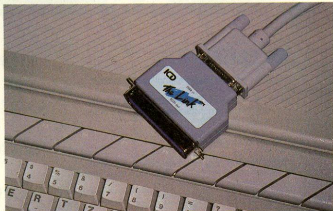
The Link: ICD-Host-Adapter in Steckergröße
